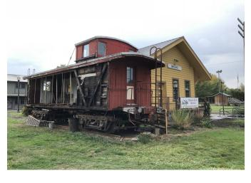
more modern times - maybe 1960 when they painted it bright red. The thick planks had rotted out underneath. The Burlington shops used a spray undercoating like the old Z Bart used on autos. So we did not know how bad until crunching thru the planks.
